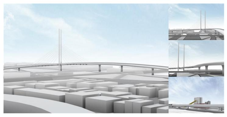
FHECOR Ingenieros Consultores carried out the study of alternatives and tender design project of two bridges for the new East-West Link in Melbourne, as requested by John Holland, Leighton Contractors and Dragados Joint Venture. They consist of two urban bridges designed to become iconic landmarks for the city: a cable statyed bridge over the East-West Link and Hoddle St. Interchange, and a tube shaped steel truss over the City Link Highway.
